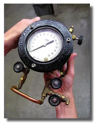
Field test kit position during field testing of backflow prevention assemblies is crucial and noted in chapter nine of the Manual of Cross-Connection Control, Tenth Edition. Not raising the gage to the appropriate elevation may result in inaccurate reading leading to prematurely failing an assembly or passing an assembly which does not meet the requirements for passing the field test.
