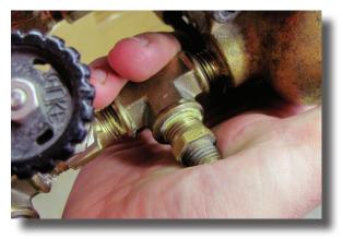
low side and bypass hoses are detached, the tester must be careful not to place their hand over the ports where the hoses would be attached.
